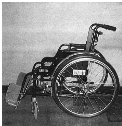
Wheelchair B Weight: 13.5 kg Wheel diameter: 22 inch Height to hand grips: 77 cm
